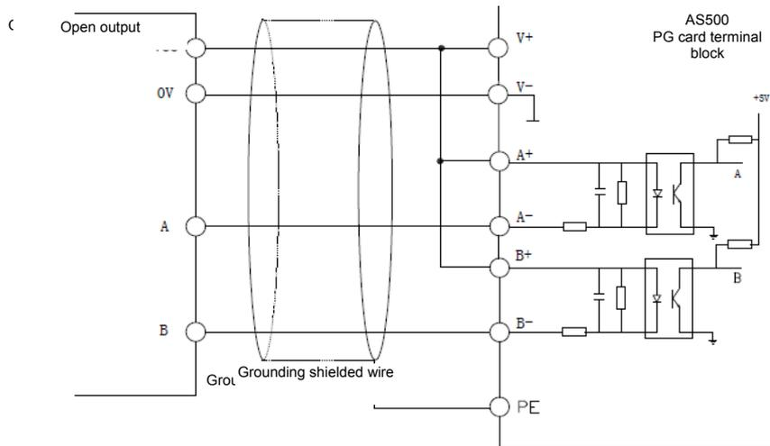
Figure 4-29 Wiring with the open collector signals of the encoder
