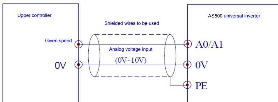
Figure 4-26 A0/A1 analog voltage signal wiring
