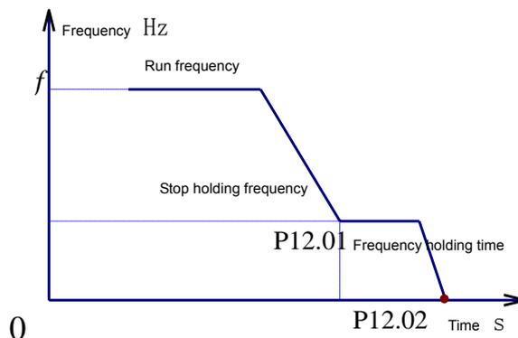
Figure 7-10 Stop holding frequency diagram
