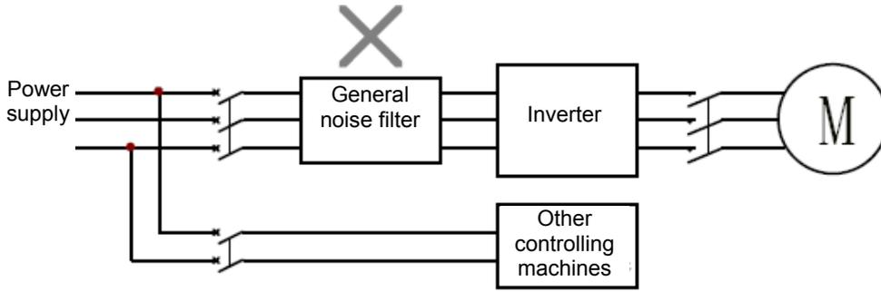
Figure 4-3 Example 1 for incorrect layout of noise filter on the power side
