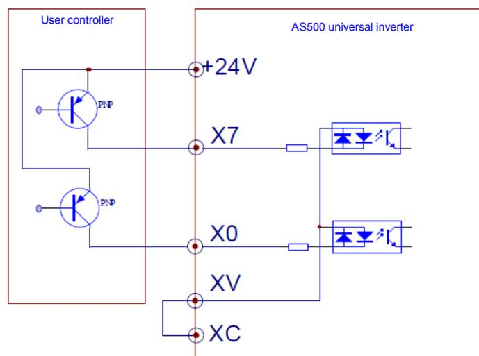
Note: take care to remove the short-circuit bar between +24 V and XV terminals, and connect the bar between XC and XV terminals.
