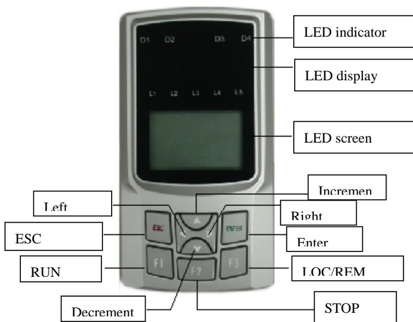
Figure 5-1 Components and their functions of the digital operator
