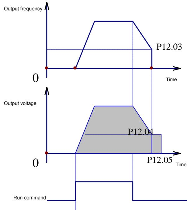
Figure 7-11 Stop DC braking diagram
