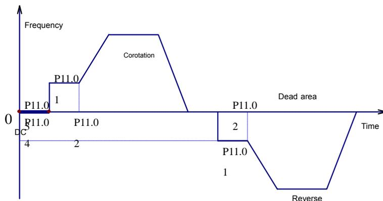
Figure 7-6 Start mode diagram of DC brake
