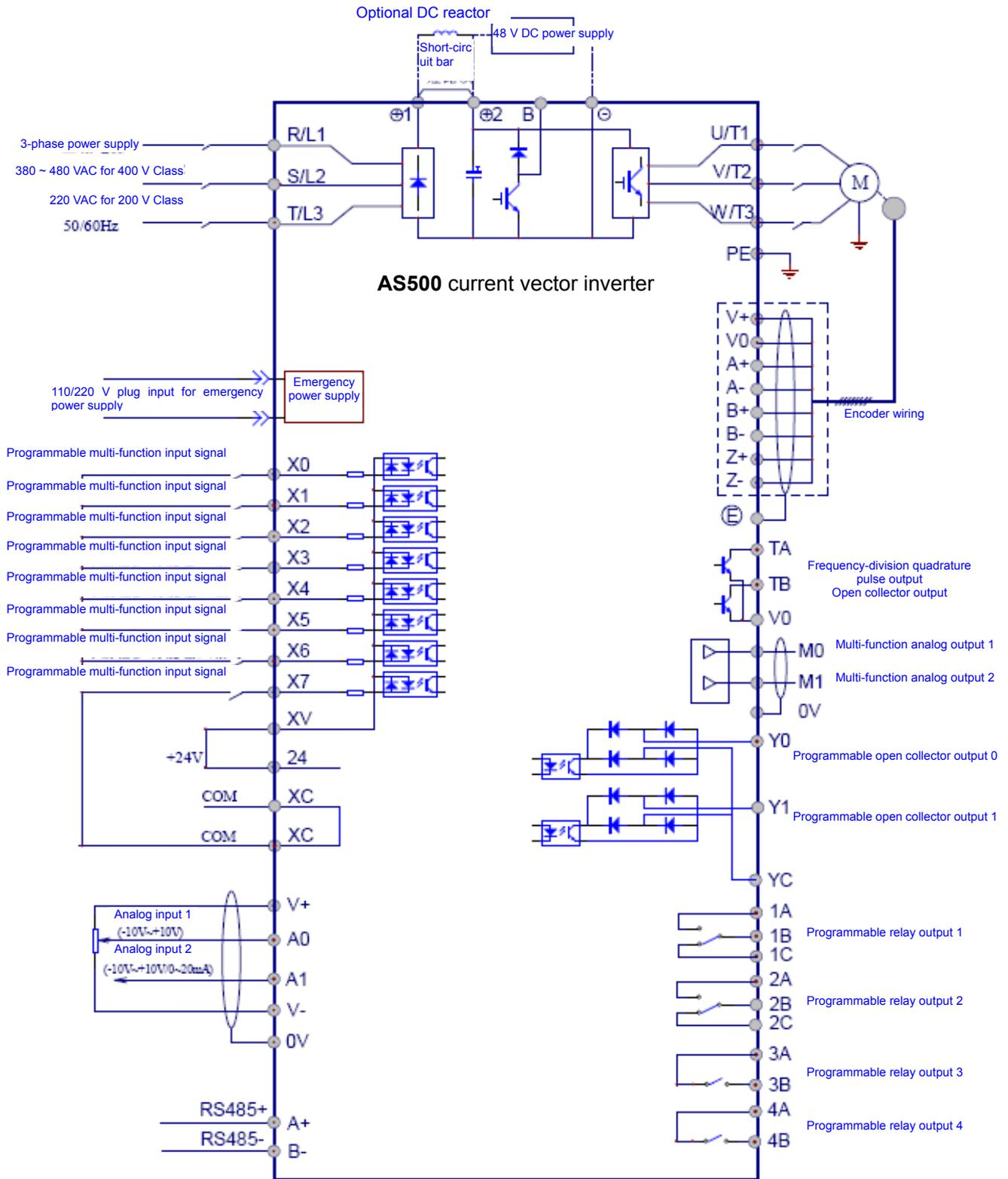
Figure 4-7 Schematic diagram 1 for terminals wiring of universal inverter (below 30kW)
