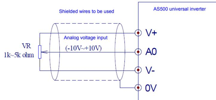
Figure 4-25 Shielded analog input wiring
