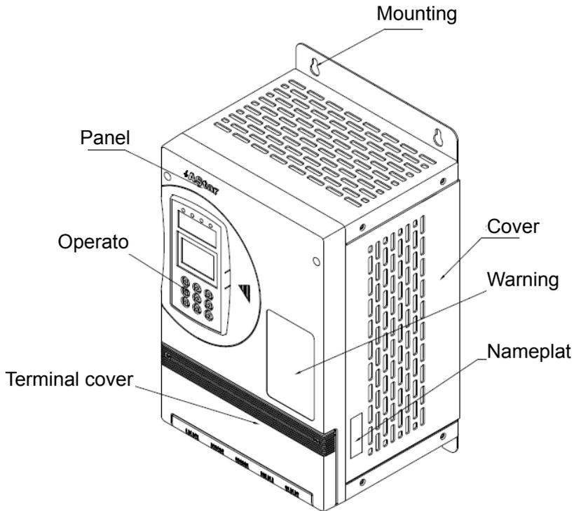
Figure 2-5 For AS500 4T07P5 and above power
