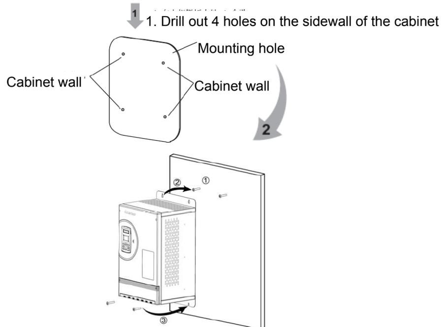
Figure 3-6 Installation order of inverter
