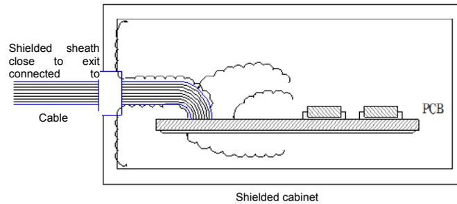
Figure A.10 Radiation restraint by connecting the cable shield with the housing
