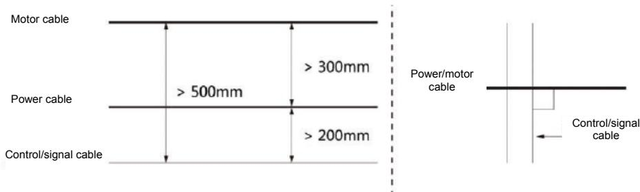
Figure 4-19 Layout 1 of main circuit wiring
