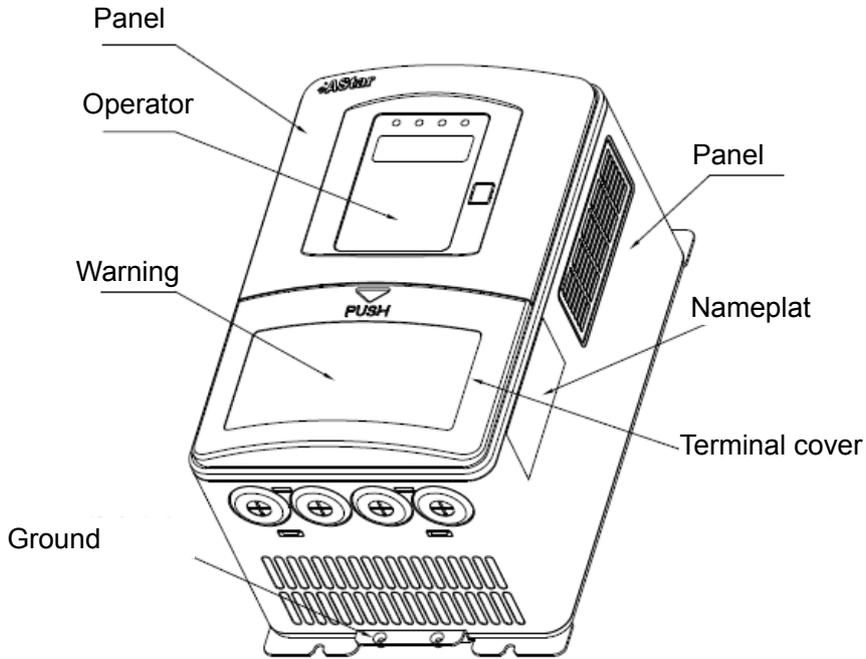
Figure 2-4 For AS500 4T05P5 and below power
