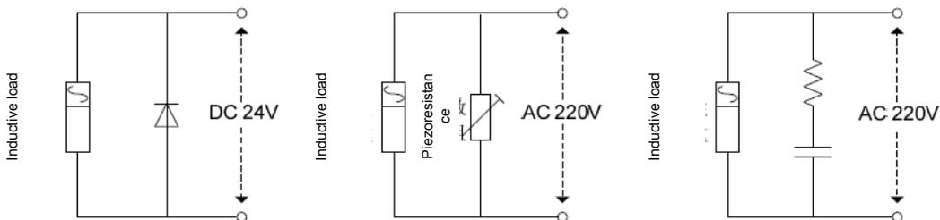
Figure 4-18 Application of surge suppressor for inductive load
