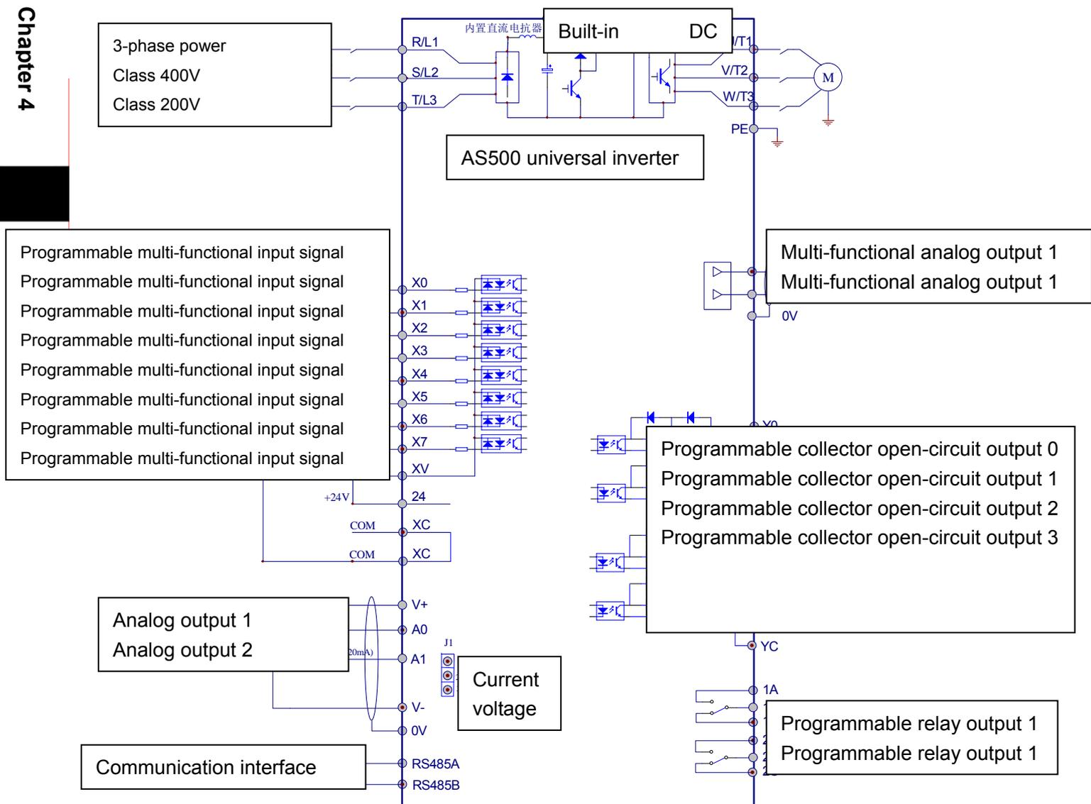
Figure 4-8 Schematic diagram 2 for inverter terminals wiring (30kW or more)
