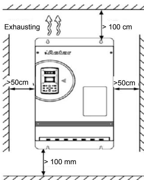
Figure 3-4 Space for installation of the inverter Figure 3-5 Space for installation of the inverter
