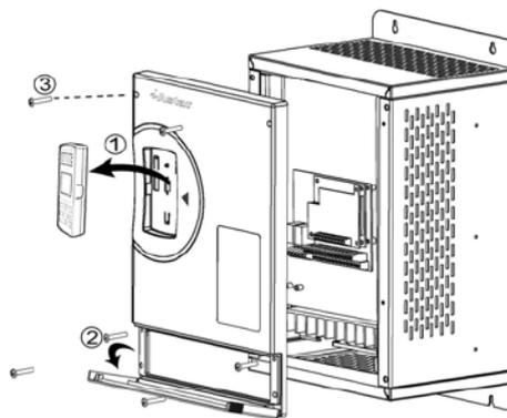
Figure 3-9 Front panel removal
