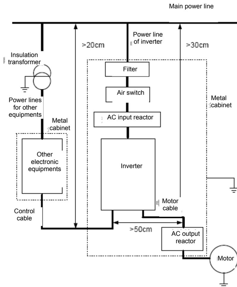
Figure A.12 Electric installation of the inverter
