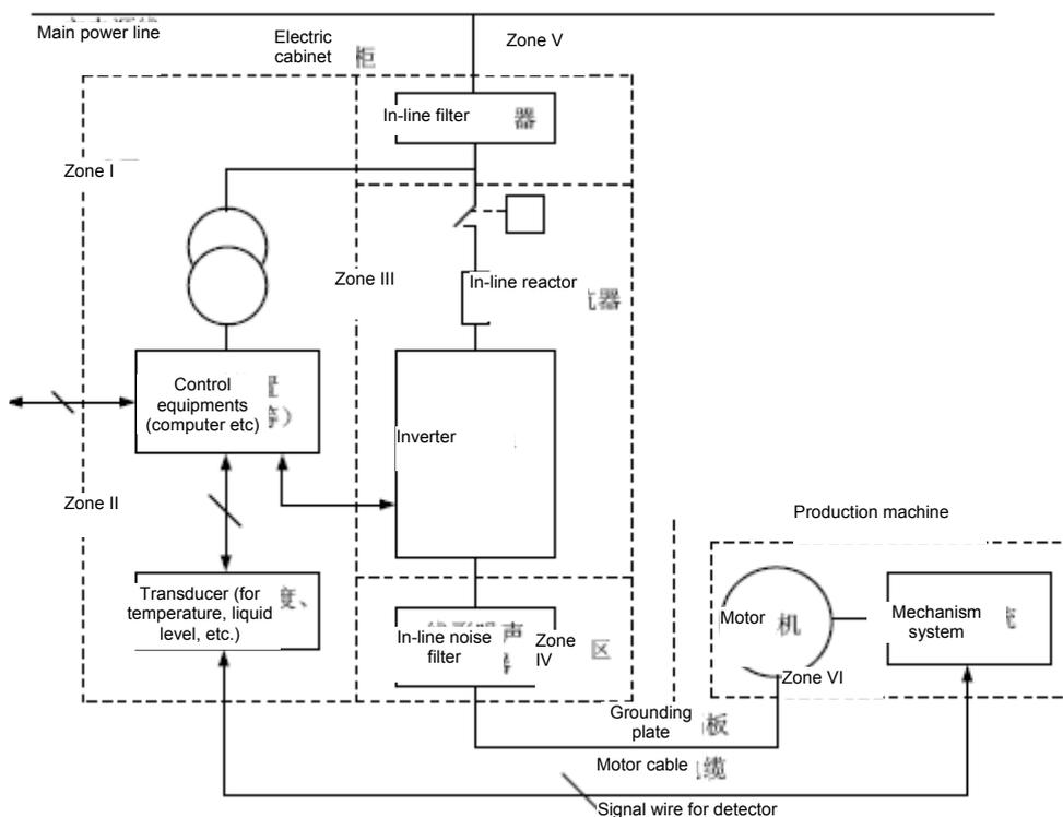
Figure A.11 EMC installation areas for the inverter
