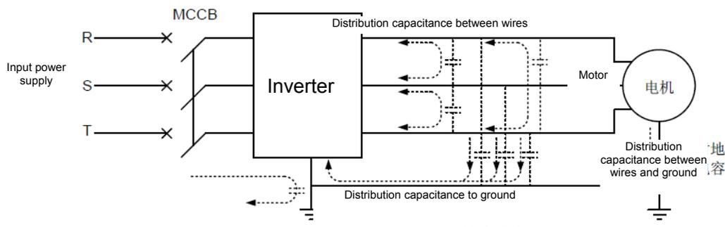
Figure A8 Leakage current path
