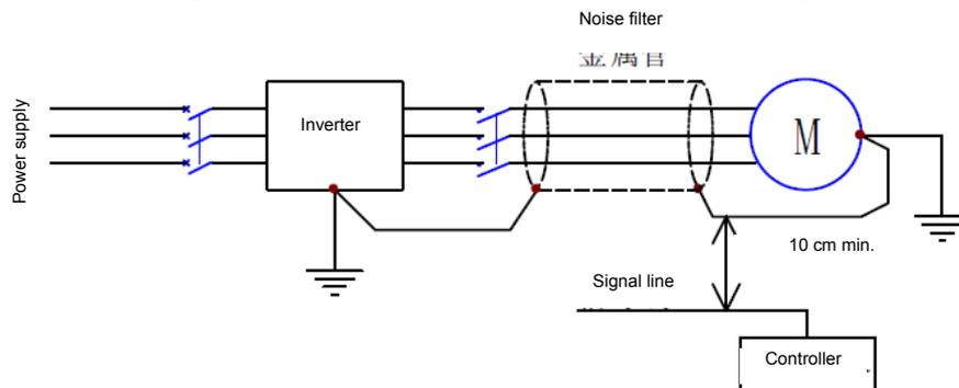
Figure 4-20 Layout 2 of main circuit wiring
