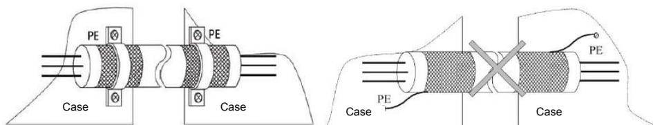
Figure 4-22 Comparison of grounding methods
