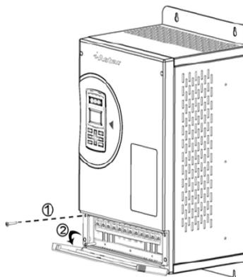
Figure 3-8 Opening the terminal cover
