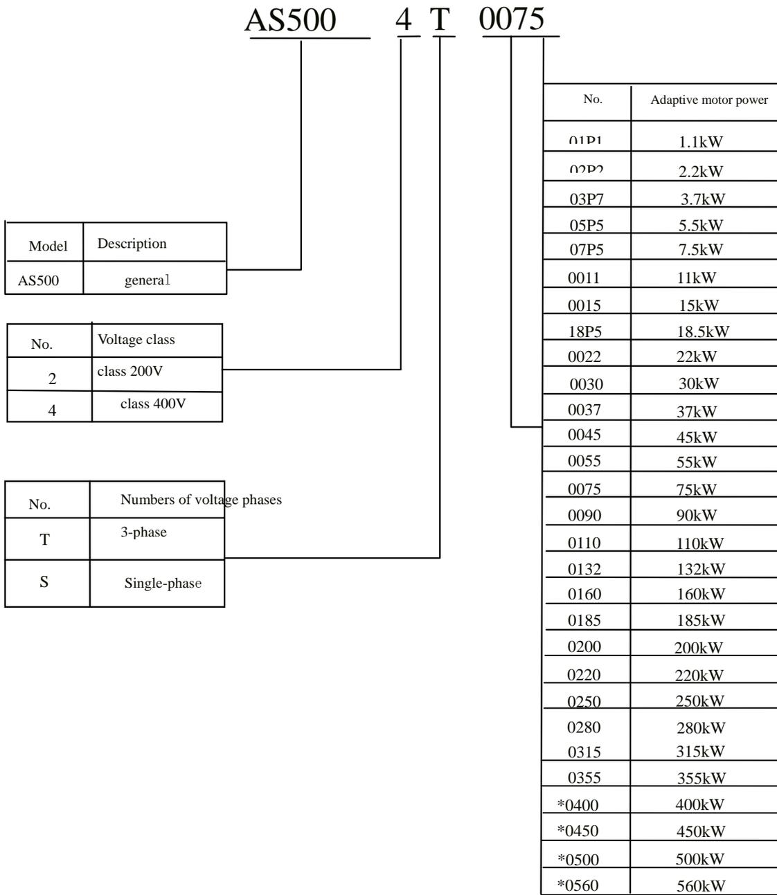
Figure 2-3 Inverter model specifications
