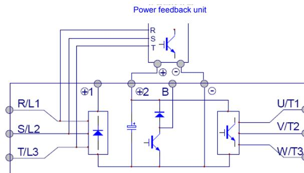
Figure 4-15 External power feedback unit
