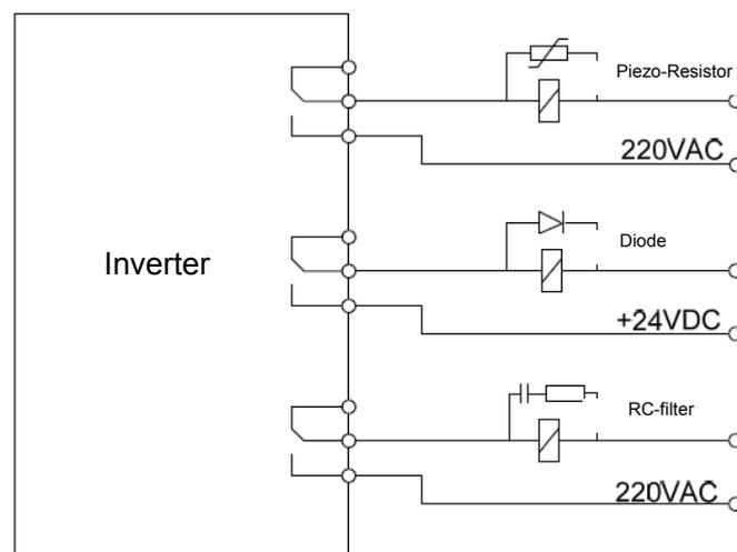
Figure A.7 Application of relay, contactor and electromagnetic brake
