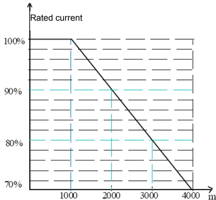
Figure 3-1 Relation between rated output current of inverter and altitude
