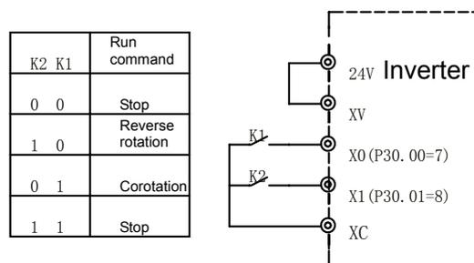
Figure 7-1 Two-wire running mode 1
