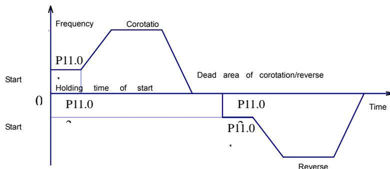
Figure 7-5 Start mode diagram of start frequency
