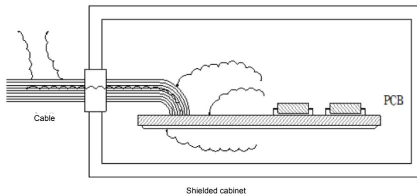
Figure A.9 Radiation from cables going out the shielded cabinet
