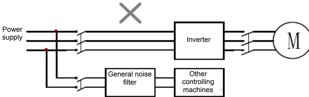
Figure 4-4 Example 2 for incorrect layout of noise filter on the power side
