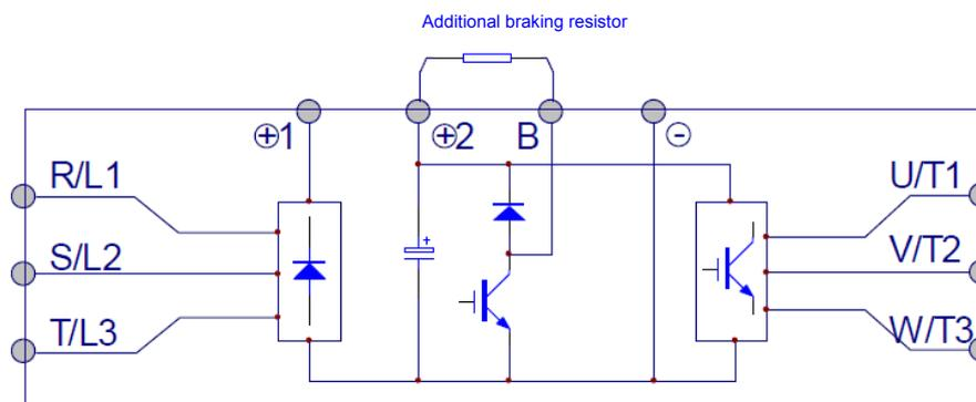
Figure 4-13 Braking resistor wiring
