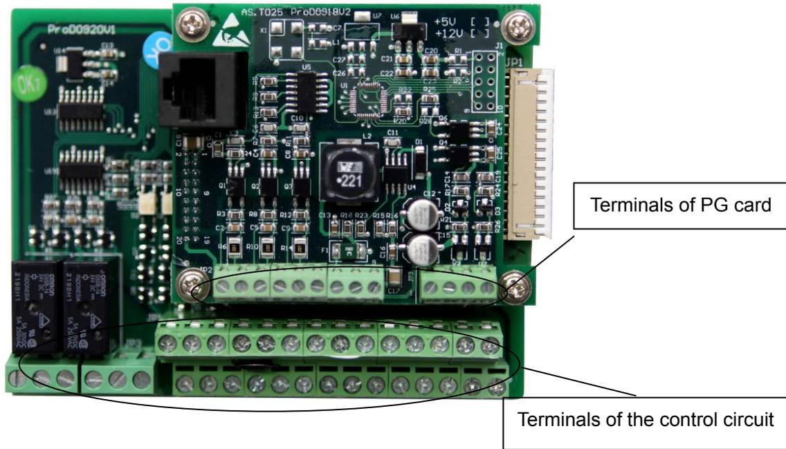
Figure 4-23 Terminals picture of the control circuit
