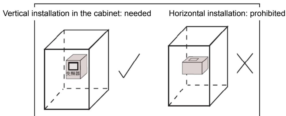
Figure 3-2 Installation orientation
