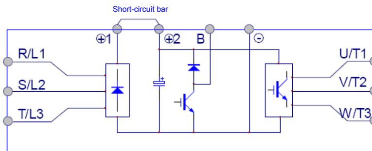
Figure 4-11 Wiring diagram of short-circuit bar
