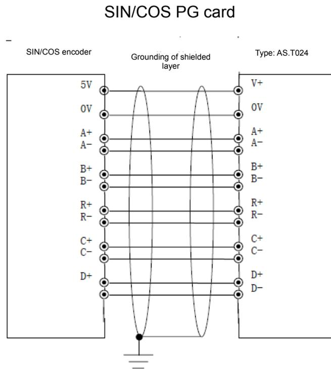
Figure 4-32 Wiring with SIN/COS differential signals of the encoder
