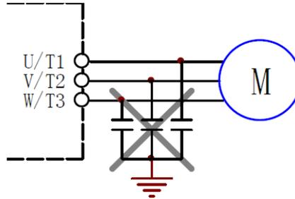
Figure 4-16 Never connect capacitor on the output side of the inverter
