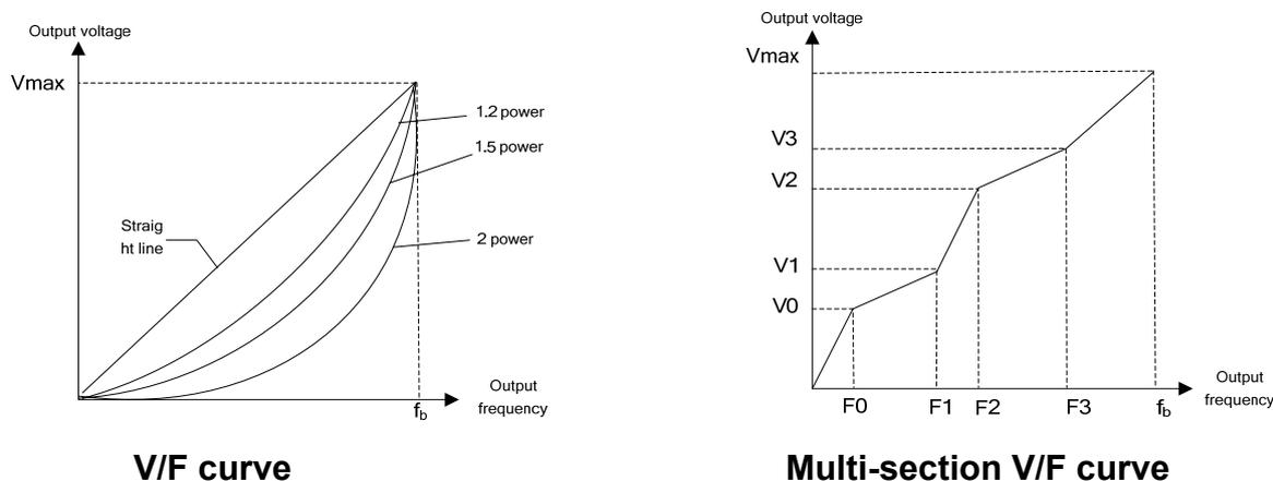
Figure 7-12 VF curve diagram
