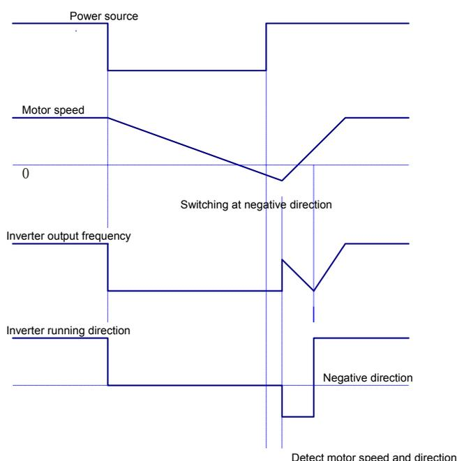
Figure 7-6 Start mode diagram of speed track
