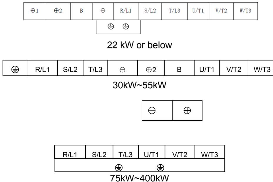
Figure 4-9 Main circuit terminals diagram
