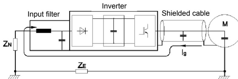
Figure 4-5 Schematic for noise current of noise filter
