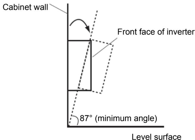
Figure 3-3 Permissible included angle for installation
