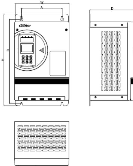
Figure 2-7 Installation dimensions of AS500 4T07P5 and above inverters
