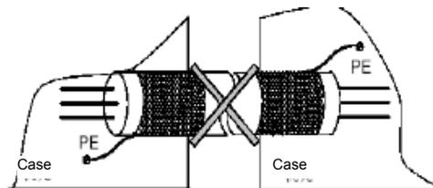
Figure A.3 Incorrect wiring to PE
