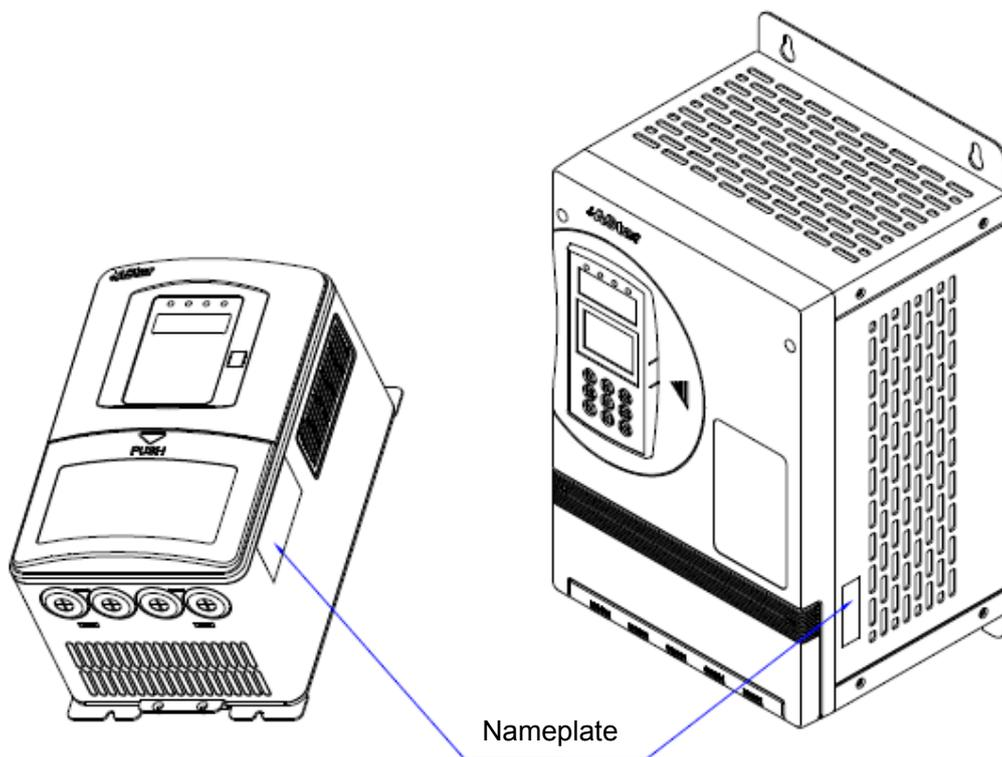
Figure 2-1 Inverter nameplate (example)
