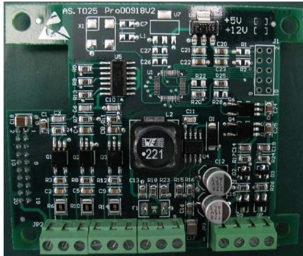
Figure 4-28 Terminal alignment of ABZ increment PG card
