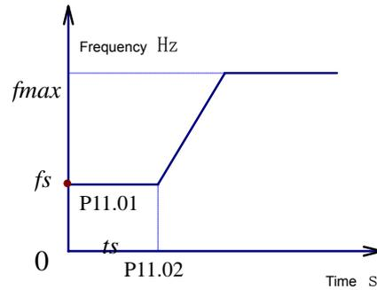
Figure 7-7 Start frequency and start time diagram
