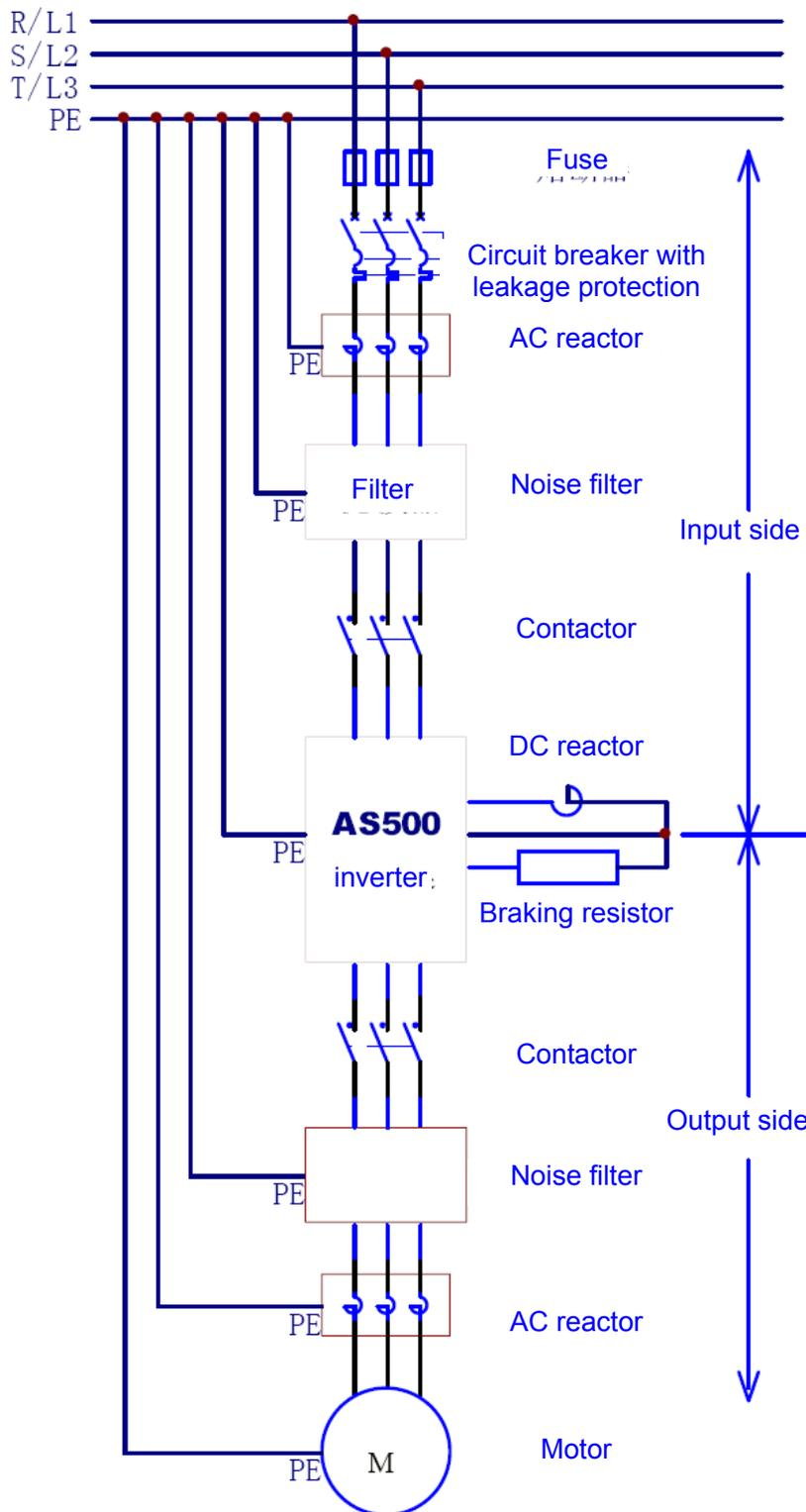
Figure 4-1 Connection diagram of the inverter and peripheral devices
