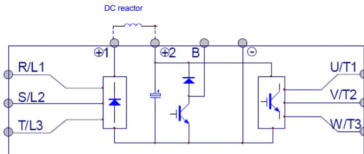
Figure 4-12 Wiring of the DC reactor
