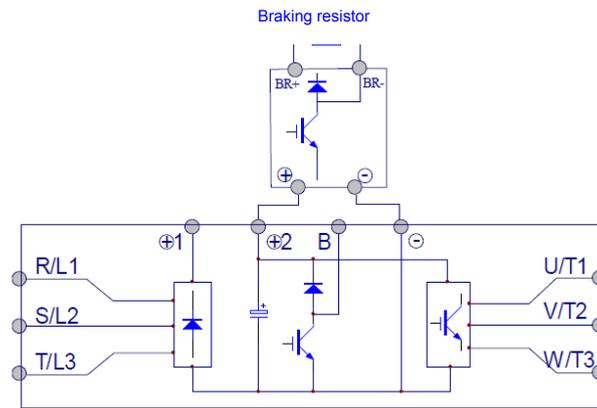
Figure 4-14 External braking unit
