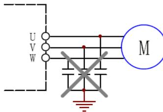
Figure 1-1 Schematic diagram for non-permission for capacitor connection at the output side of the inverter
