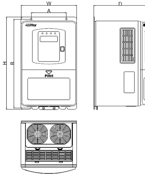
Figure 2-6 Installation dimensions of AS500 4T05P5 / 2T07P5 and below inverters
