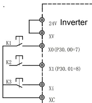
Figure 7-3 Three wire running mode 1
