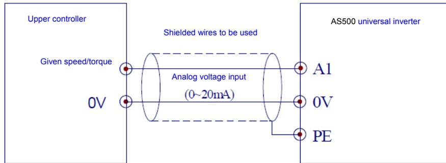
Figure 4-27 A1 analog current signal wiring
