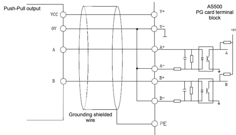
Figure 4-30 Wiring with the Push-Pull signals of the encoder
