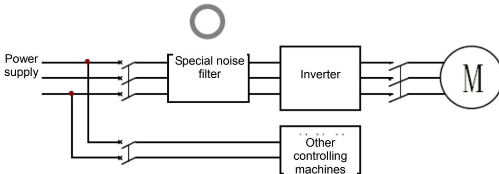
Figure 4-2 Proper layout of noise filter on the power side
