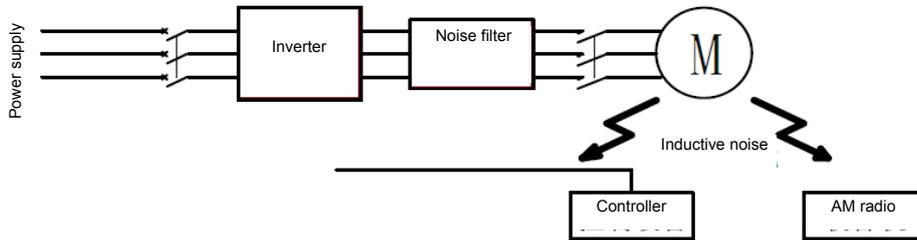
Figure 4-18 Connection of noise filter on the output side of the inverter
