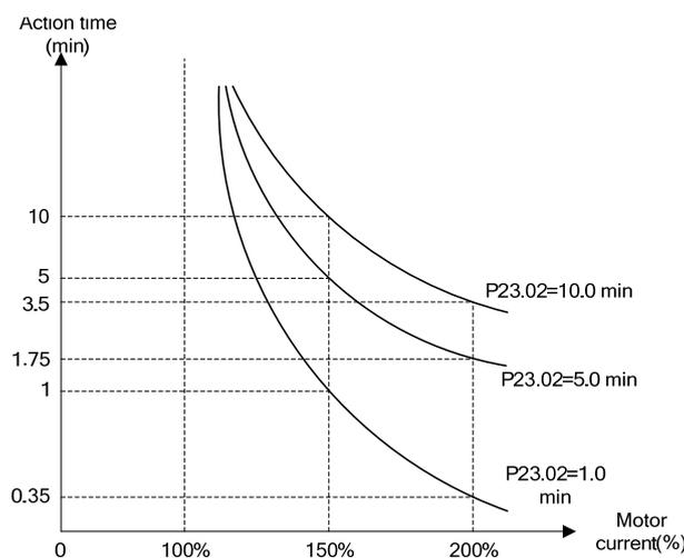
Figure 7-14 Motor overload protection feature curve (constant-torque)
