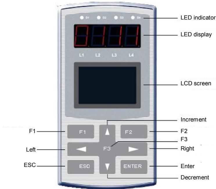
Fig- 5.1 Components and their functions of the digital operator
