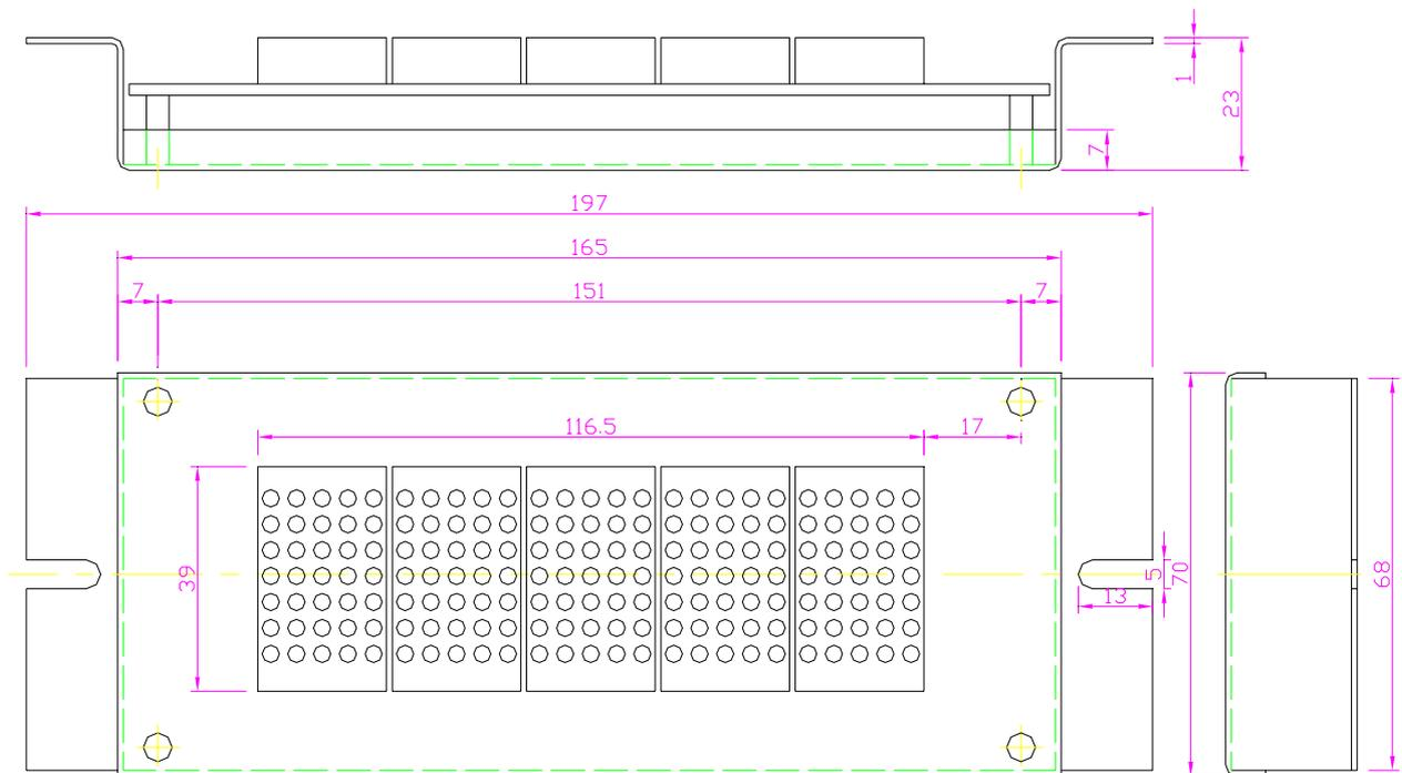
Fig. 2-9 (B) Mounting Dimensions of SM-04-HRC
