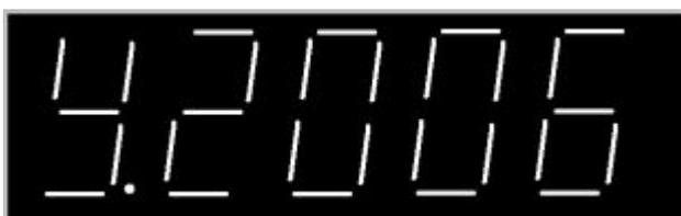
The meaning of figure above is 2000 year. "Y" is the abbreviation of Year. When modification required, press "Enter", the lowest order of digit begins to flash. Use the "left" and "right" buttons to select the position where
