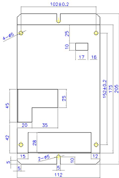
Fig. 2-12 (B) Mounting Dimensions of SM-04-UL
