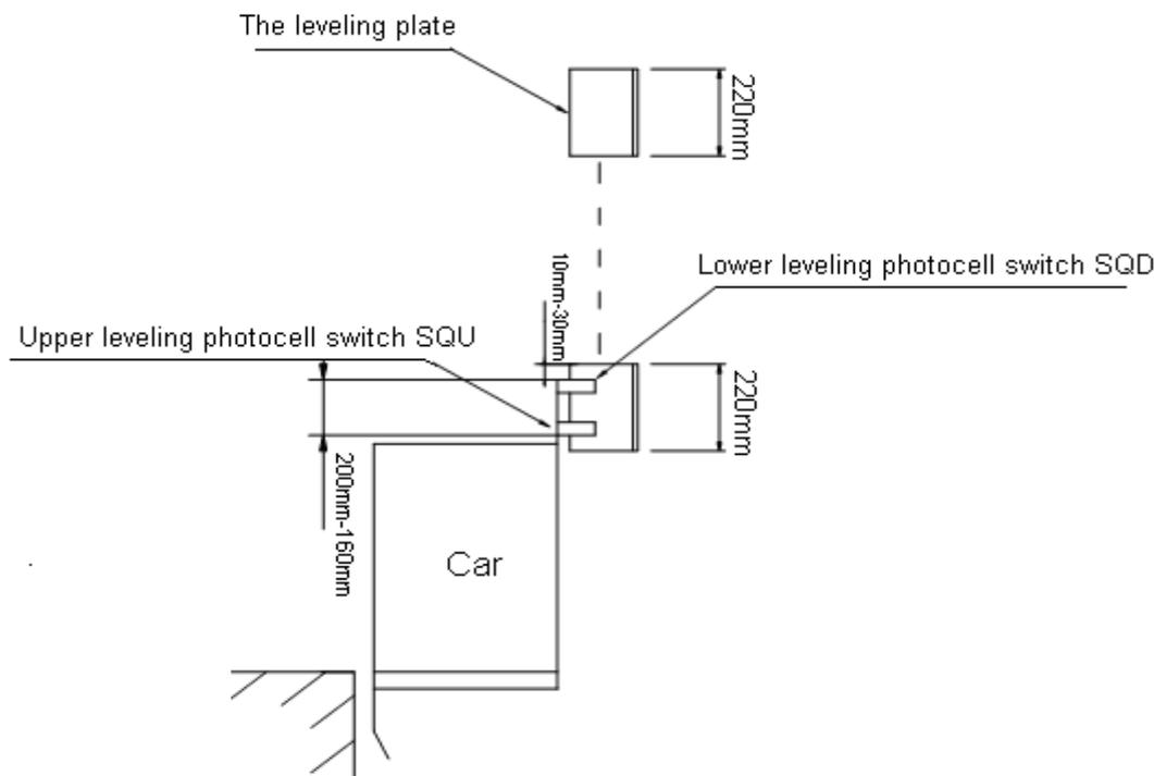
③ The leveling plates of every floor should be in alignment with the inductor by the central line for better leveling performance after recording the floors.
