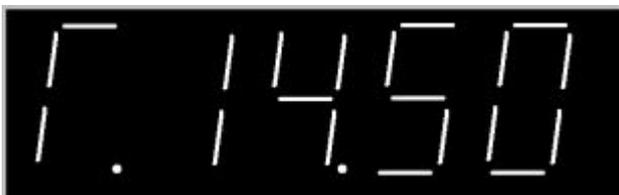
Time: The meaning of figure above is that the fault occurs at 14:50. "T "is the abbreviation of Time.
