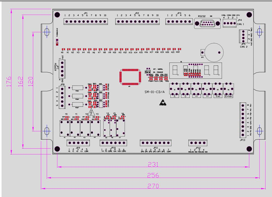
Fig. 2-2 (B) Mounting Dimensions of Master Control Board
