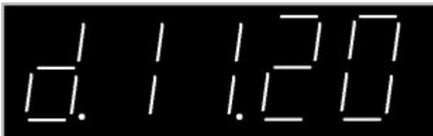
Date: The meaning of figure above is that the fault occurs on Nov. 20. "d" is the abbreviation of Day.
