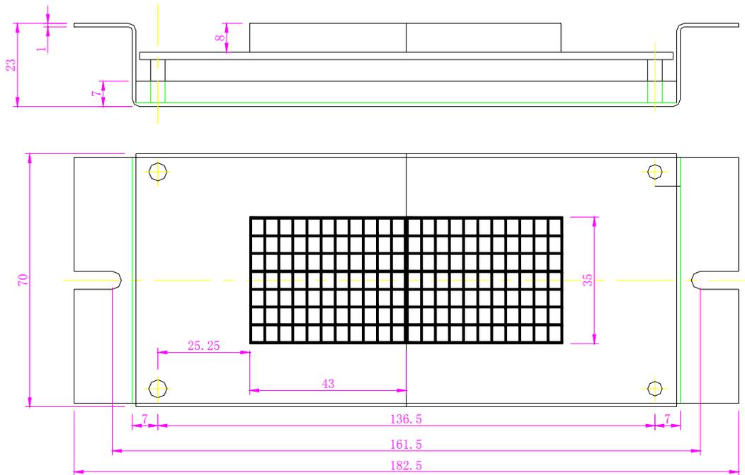
Fig. 2-10 (B) Mounting Dimensions of SM-04-HSC
