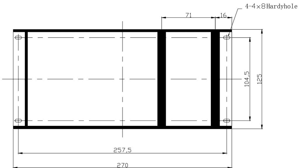
Fig. 2-5 (B) Mounting Dimensions of Car Call Board
