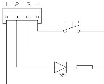
Fig. 2-6 Connection of Door Open/Close Buttons & Indicators
