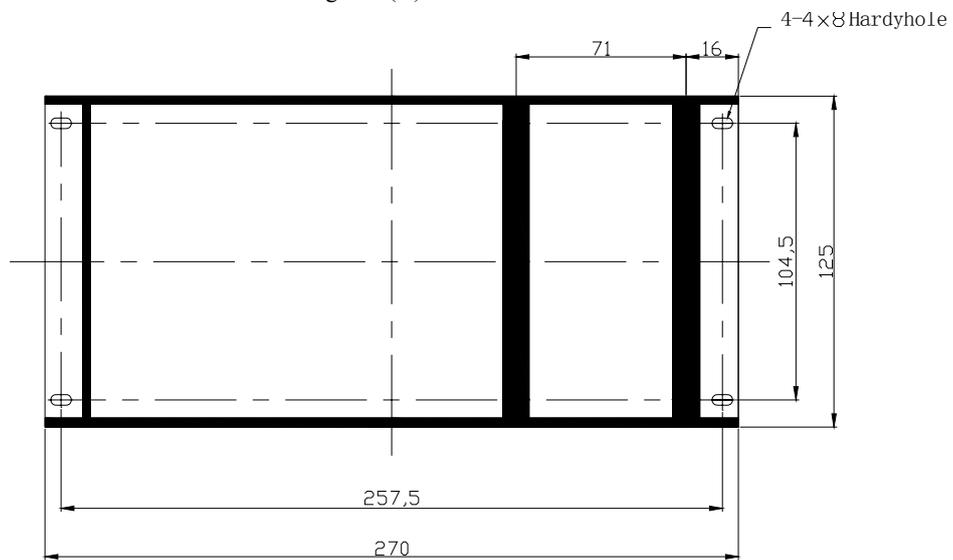
Fig. 2-3 (B) Mounting Dimensions of Car Board
