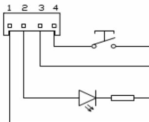
Fig. 2-4 Connection of Door Open/Close Buttons &amp; Indicators
