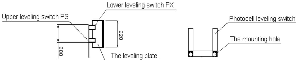
**(1) When using magnetic leveling switches**
