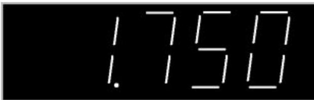
This menu shows the current running velocity of elevator in m/S. The current velocity is 1.75m/S, as it shows above.
