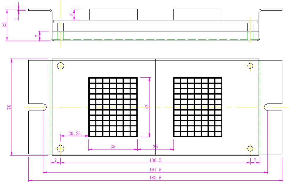
Fig. 2-8 (B) Mounting Dimensions of SM-04-VSC
