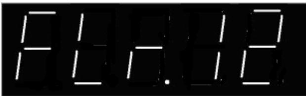
Floor: The meaning of figure above is that the fault occurs on 12<sup>th</sup> floor. "Flr" is the abbreviation of Floor.
