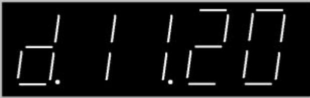
The meaning of figure above is Nov 20. "d" is the abbreviation of Day. When modification required, press "Enter", the lowest order of digit begins to flash. Use the "left" and "right" buttons to select the position where modification required, the chosen digit begins to flash. Then use the "up" and "down" buttons to modify digit, press "Enter" to affirm modification.
