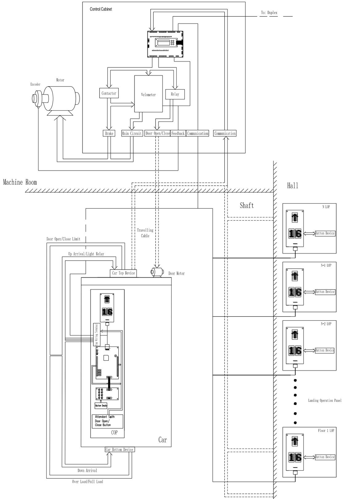
Fig. 2-1 Configuration of Serial Control System
