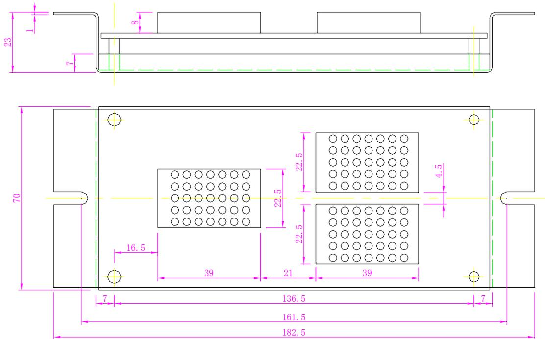
Fig. 2-7 (B) Mounting Dimensions of SM-04-VRF
