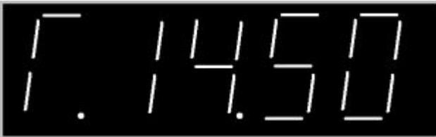
The meaning of figure above is 10:50. "T" is the abbreviation of Time. Notes that due to the limit of seven segment code, the "T" in CD/A is shown as above. When modification required, press "Enter", the lowest order of digit begins to flash. Use the "left" and "right" buttons to select the position where modification required, the chosen digit begins to flash. Then use the "up" and "down" buttons to modify digit, press "Enter" to affirm modification.
