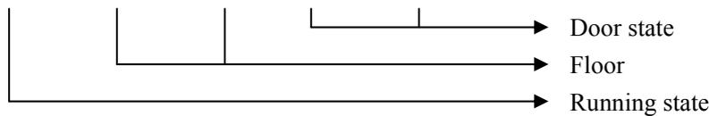
In this menu, you can see the basic states of elevator, including running state, current floor and door state. During the running state:
