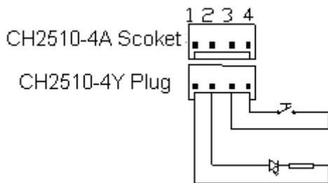
Fig. 2-13 (A) Connection of the Push Button
