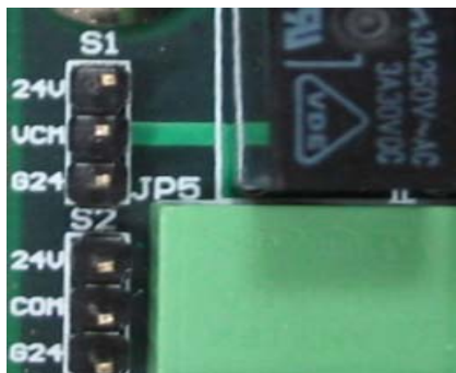
Fig 3-16 diagram of Wiring of S1、S2 jumpers (Type A1)
